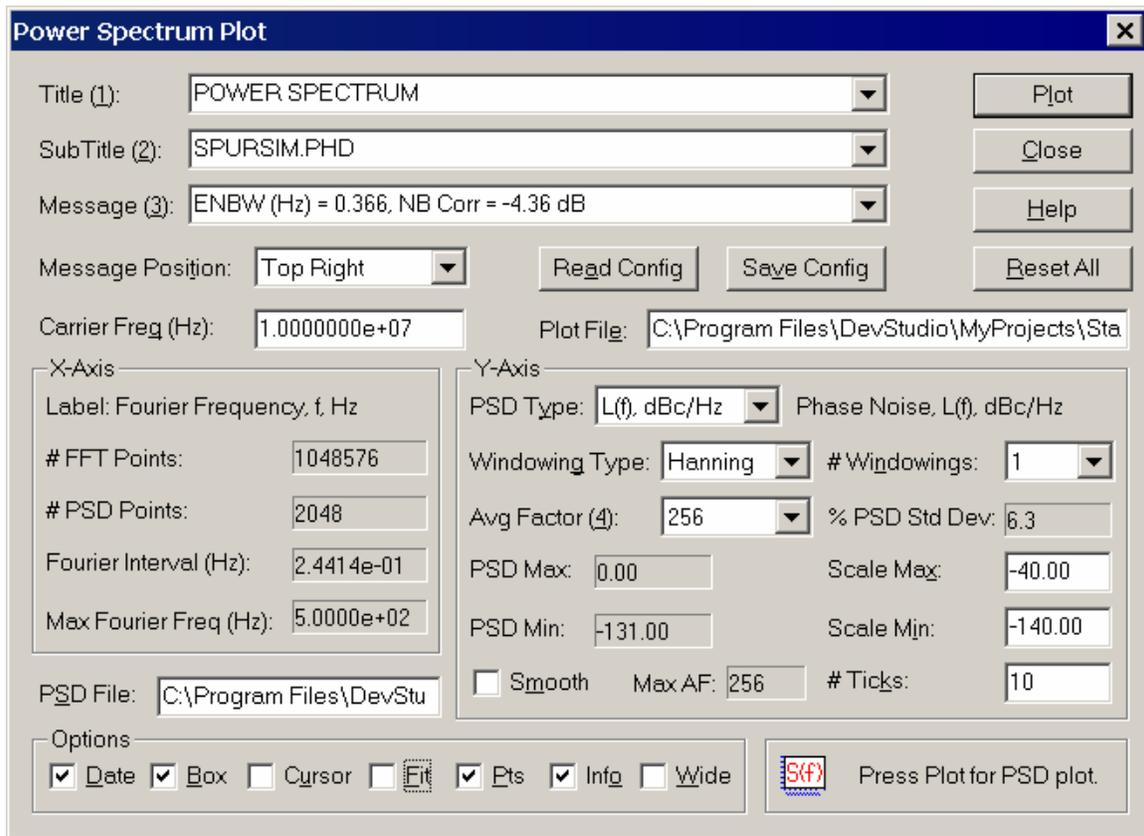
The resulting  $L(f)$  PSD plot is shown below with one Hanning window and an averaging factor of 256. Note the ENBW and narrowband log correction factors shown in the message display.
